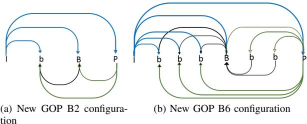
Fig. 2. New GOP configurations. (a) Extended GOP configuration by removing a **b** frame. (b) Extended GOP configuration by adding a **b** frame.
